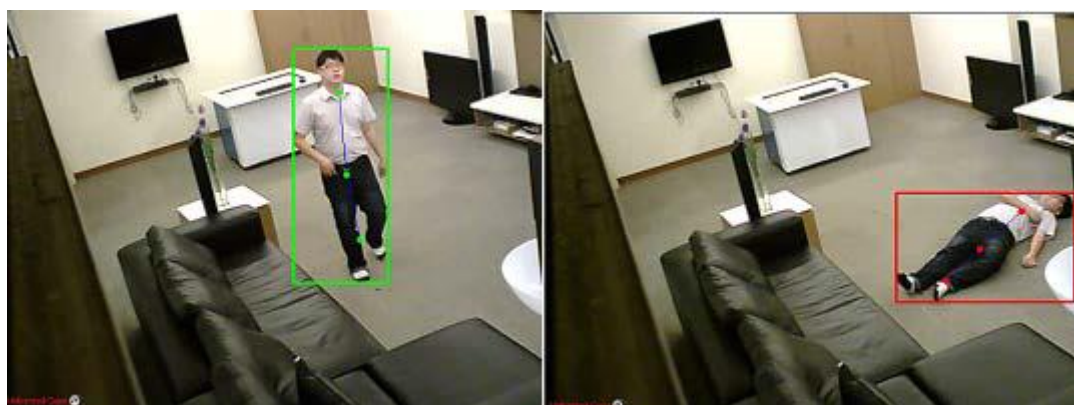
Figure 18: Visual examples of a normal detection (green blob on the left) and a fall detection (red blob on the right).
