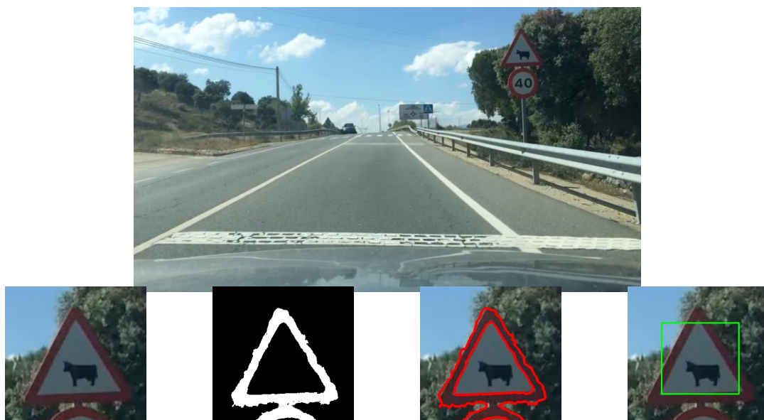
Figure 10: Traffic signs detection and recognition example. Input image, signal detection, color segmentation, edge extraction and sign recognition.
